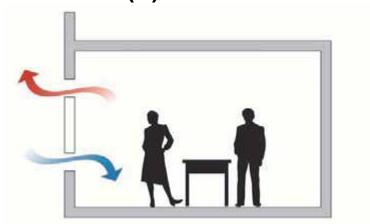
Single sided ventilation – via opening window, drawing air in by natural convection currents. This air will typically mix with warm air rising from radiators, etc.
